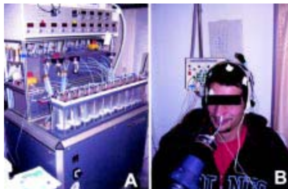
Figure 1: A. Computer-controlled olfactometer suited for separate/combined application of 6 different odorous stimuli (OM6, Burghart, Wedel, Germany). B. Intranasal application of odorous stimulation and EEG recording.
