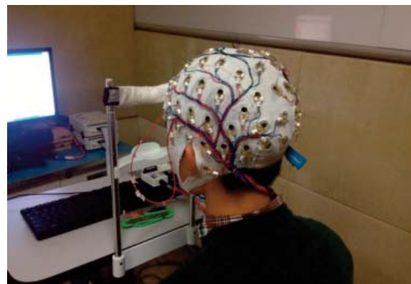
Figure 2: The 64 Ag/AgCl scalp electrodes mounted on the elastic cap (Easycap GmbH, Herrsching-Breitbrunn, Germany). After wearing the Easycap, subjects placed their chins on a chin rest and viewed the central display horizontally with the amblyopic eye or the nondominant eye (controls).
