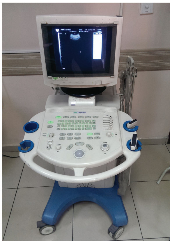
Figure 1: Ultrasound device CHISON 8500 with a 3.5 MHz curvilinear transducer which is used for bedside ultrasound in the emergency department.
